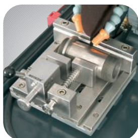
Stainless steel clamping devices and T-slotted table
