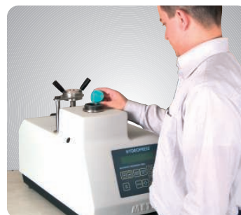
Electro-hydraulic pump and preprogrammed moulding sequences allow a smooth and comfortable operation.
